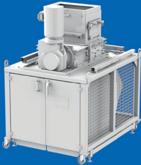
Chip reducer ZVD 400-J on a frame for volume reduction
